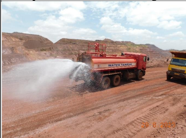
Dust suppression on Mine Benches with Hydraulic water sprinkler system
