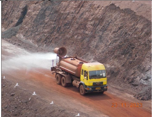
Truck Mounted Dry Fog dust suppression system
